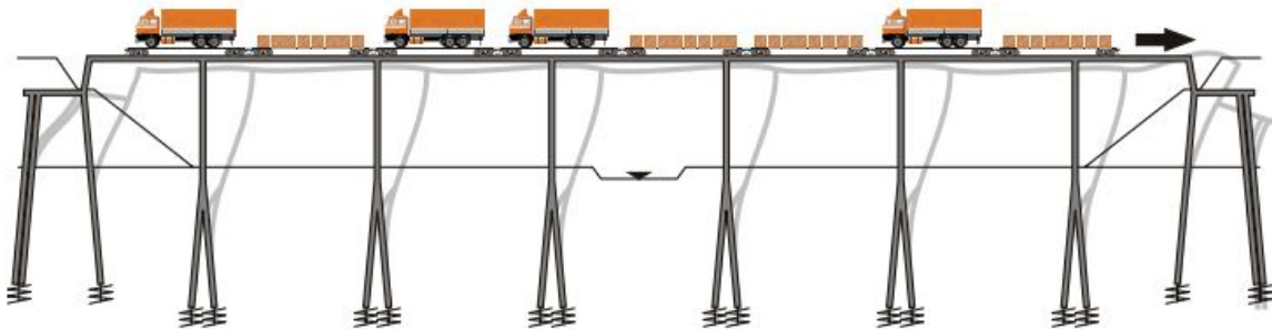
Structure deformed due to railway braking force
