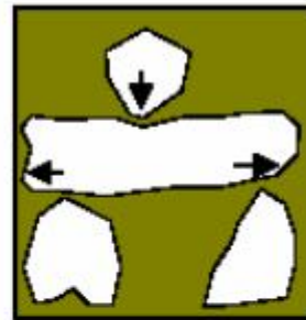
Cracked rock beam
