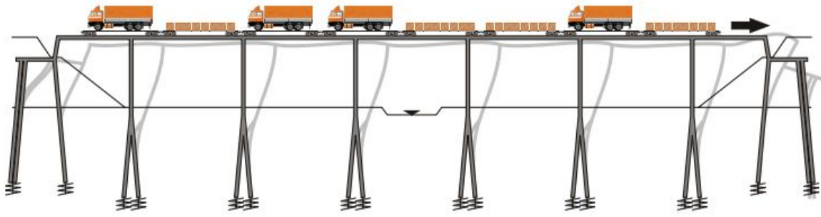
Structure deformed due to railway braking force
